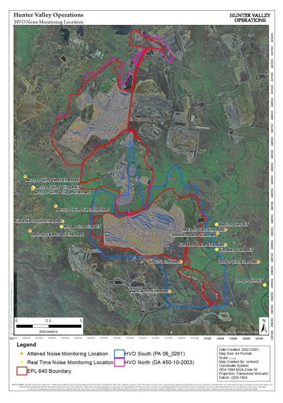
Figure 16 - Noise Monitoring Location Plan
